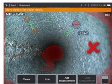
Incorrect cursor placement identified with 3D Point Cloud
